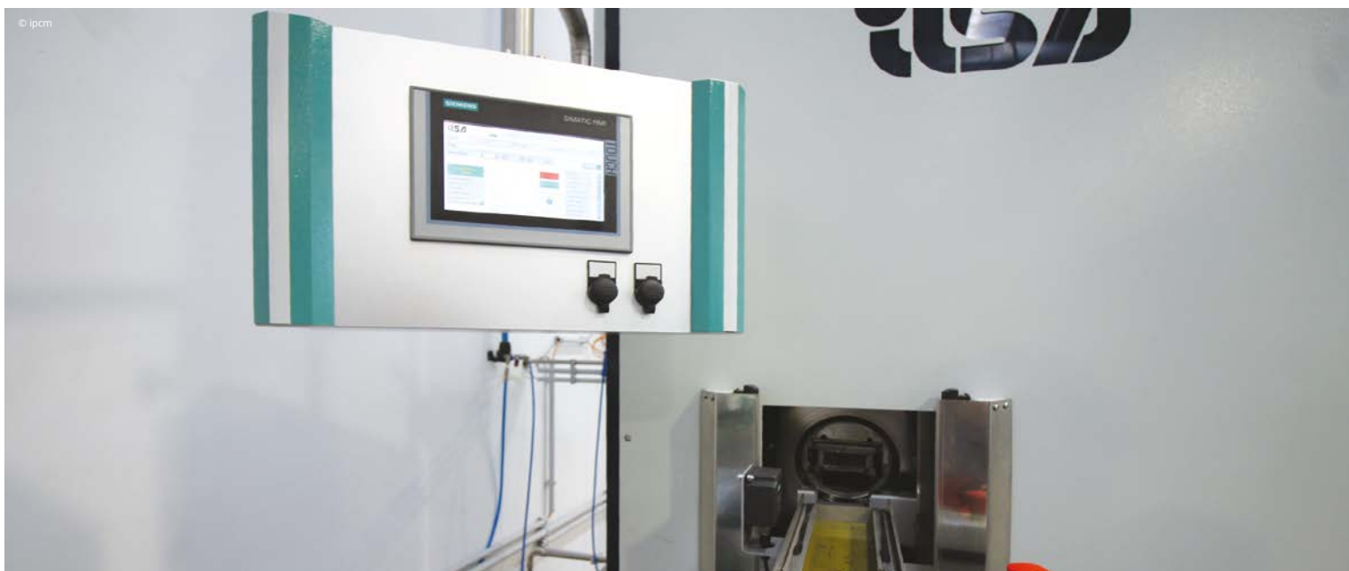
The touch screen panel of the cleaning system.
